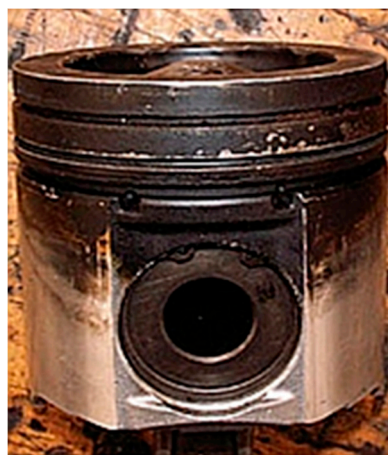
Figure 1. Effects of the “wet stacking” phenomenon [5].
